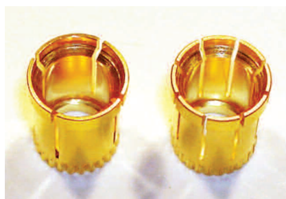
▲ Fig. 1 The un-plated industry-standard tines (right) and the un-plated Times new design (left).
